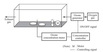
Fig. 1 Schematic of experimental apparatus
